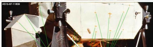
Apollo 15 LEM held together by masking tape
